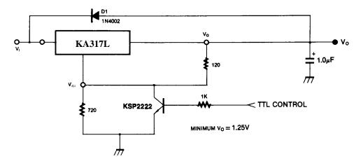
D1 protects the device during an input short circuit.
